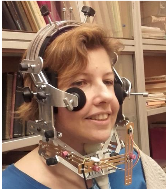
Fig. 1: Ultrasound stabilization helmet with the fixed ultrasound transducer and lip camera (in the front of the lips).
