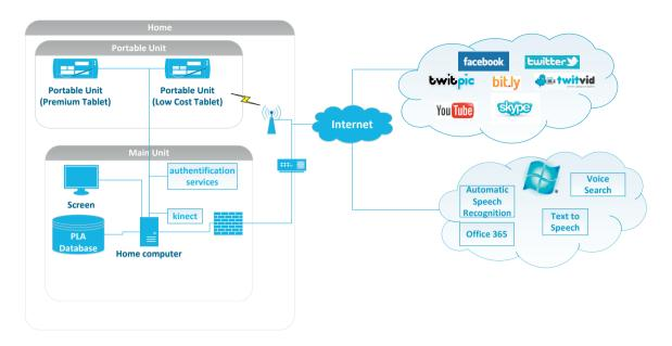
Figure 2: The architecture of the PLA.
