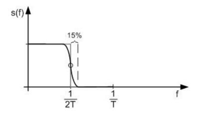
so, the bandwith of the QAM:  $2 \cdot \frac{1}{2T} 1.15 = 8MHz$ , where the symbol rate is 1/T.
